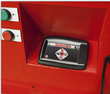
Touch screen controller
