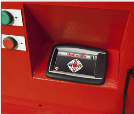
Touch screen controller
